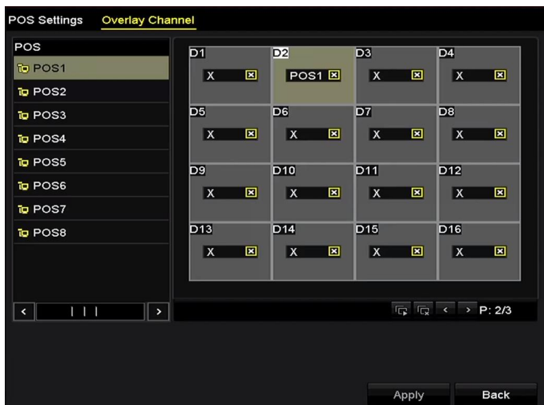
Figure 9-11 Overlay Channel Settings
